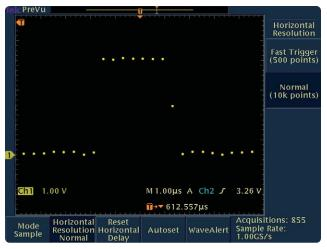
Figure 12. Zooming-in on the burst shows just a single digitized point on the runt pulse due to insufficient sample rate and memory depth (note: dots have been enhanced for clarity)
