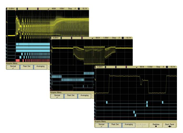
Figure 7. Motor drive signal start-up sequence with digital control signal triggering and various levels of zoom to reveal "runt" pulse using Agilent's 6000 Series MSO
