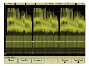
Figure 3. Full frame of composite video displayed on Agilent's 60000 Series scope
