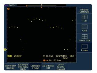
Figure 6. Zoomed-in display of a single line of video using the Tek TDS3000 Series scope (note: dots have been enhanced for clarity)
